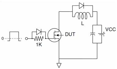
3) Switch Time Test Circuit
