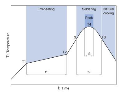
Preheating Soldering Peak Temp. Temp. Temp. Time Time Time T1 T2 T4 t3 T3 150°C 180°C 60 to 120s 230°C 245°C 40s max. 5s
